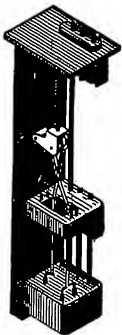
FIG. 30.—SYSTEM AS IN FIG. 29, BUT NOT SUBMERGED AND NOT CARRYING CURRENT, USED TO INDICATE THE MOVEMENT OF THE HOT WIRES
